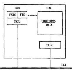
SFM = Secure File Manager IFS = Isolated File System FARM = File Access Reference Monitor FIG = File Integrity Guarantor --- = Logical channel between FIG and IFS
