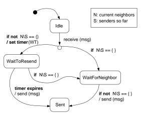
Fig. 1. State transition diagram of proposed algorithm.
