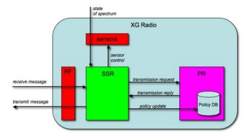
Figure 1: XG architecture. The small boxes are hardware components. The Policy DB is simply a set of policies. The SSR is a radio component that exploits transmission opportunities. This is one of many possible architectures for using our policy language.
