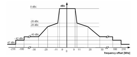
Figure 2: DFS transmit spectral powermask.
