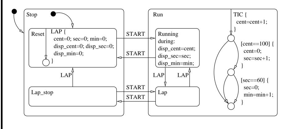
Example test goals: generate input sequences to exercise Lap\_stop to Lap transition, or to reach junction at bottom right
