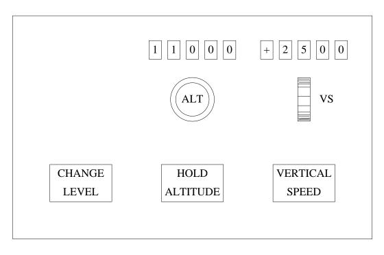
Fig. 1. The Guidance Control Panel
