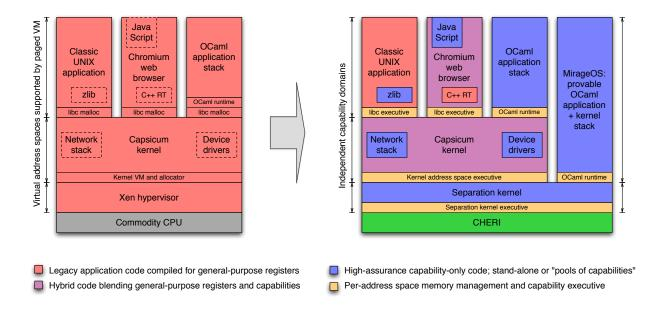
Figure 1: CTSRD proposes a *hybrid* view of the world, in which commodity page-oriented virtual memory system elements are combined with a capability system world view. Commodity applications such as Chromium will be able to exploit "pools of capabilities" — subcomponents that rely on stronger hardware protections — while allowing other portions of the applications to use lower-assurance models.
