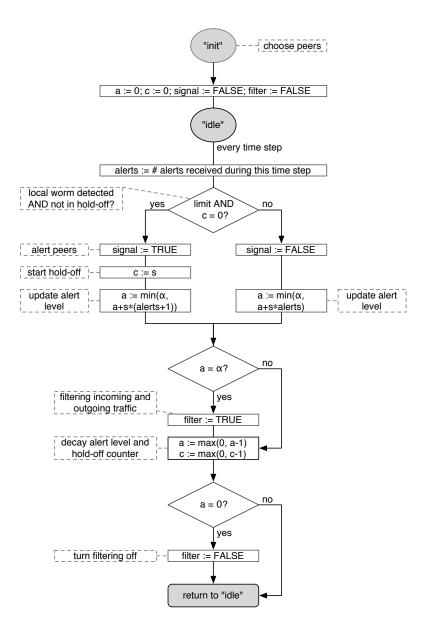
Figure 1: Flow diagram of group-based defense algorithm
