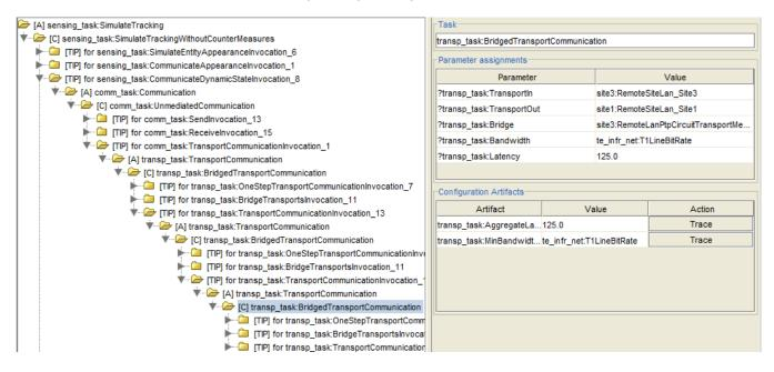
Figure 11: Result dialog showing 125 ms artifact for the partial path between Site-1 and Site-3.
