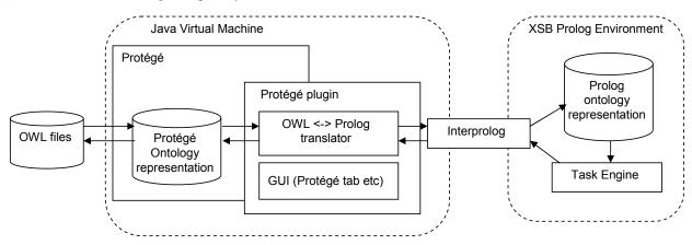
Figure 4: Implementation architecture. The new components are the Protégé plug-in and task engine. As shown by arrows, results from the task engine can be translated all the way back to OWL files.
