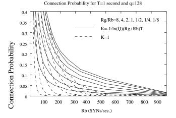
Figure 1: Connection probabilities for high ratios of spoofed SYNs
